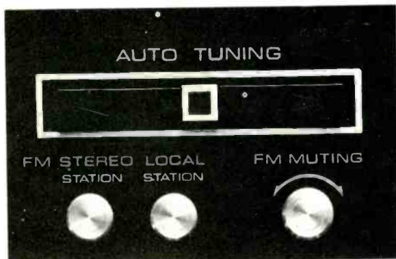
Front-panel automatic tuning controls.
