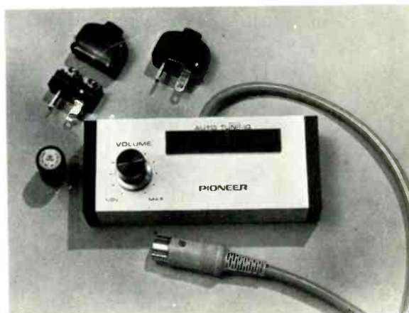
Speaker plugs (top), CdS unit (left), remote unit
