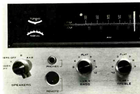
Front-panel detail showing jack for remote unit
