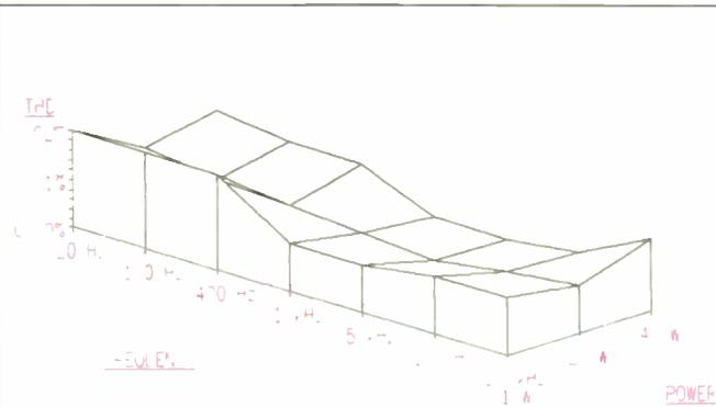
**Fig. 9—THD vs. frequency for three power levels.**
