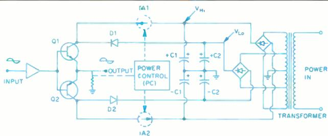
Fig. 1—The DPD (Dynamic Power on Demand) circuit.
