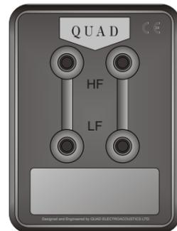
Quad crossover networks separate the treble and bass networks into two distinct sections, each connected by a dedicated pair of terminal posts. This enables the treble and bass components to be separately driven for optimum performance. The upper pair of terminals is connected to the treble network and the lower pair to the bass network.
