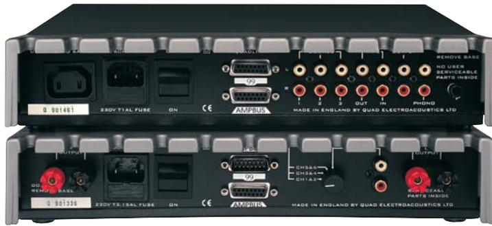
The 99 Pre-amplifier has an intelligent control system to communicate with all components connected via the 'Quad-Link' connector.
