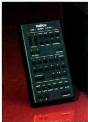
Because it also controls other Revox components, the B205 remote unit has more buttons than the B215 tape deck.
