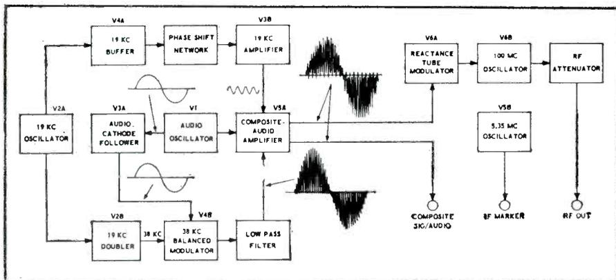
Fig. 2. Block schematic of Heathkit Multiplex Generator.
