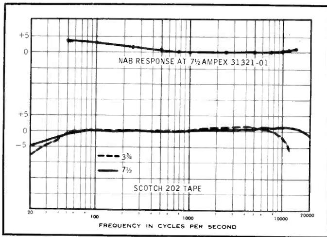
Figure 4. NAB playback and overall record/playback response of the ReVox G-36.
