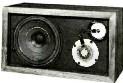
Fig. 1—AR-3a speaker system. Three speakers are revealed when front grille is removed.
