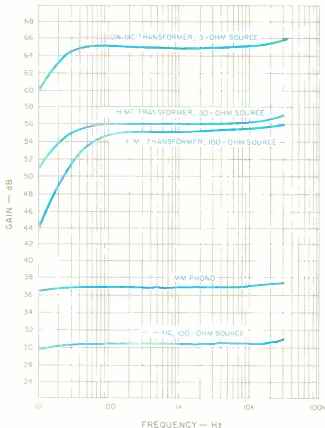
Fig. 3—Gain vs. frequency for the various phono inputs of the C-2301.
