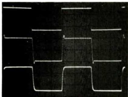
**Fig. 8—Response of B-2301 to 20-kHz square waves at various signal levels into 8-ohm loads. Top: 1-watt output; scale is 1 V per div. Middle: Clipping; scale is 50 V per div. Bottom: Below clipping; scale is 25 V per div. Time base is 10  $\mu$ S per div. for all.**
