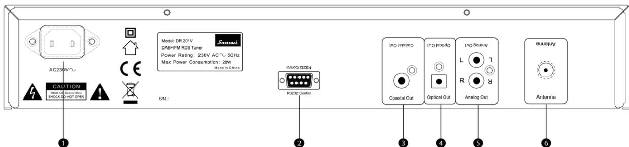
1. Power cable inlet: Plug in the supplied power cable here.
