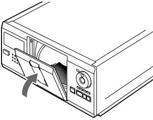
The rotary table turns and the disc slot at the loading position is set to the playing position. Always close the front cover except when you insert or remove discs.
