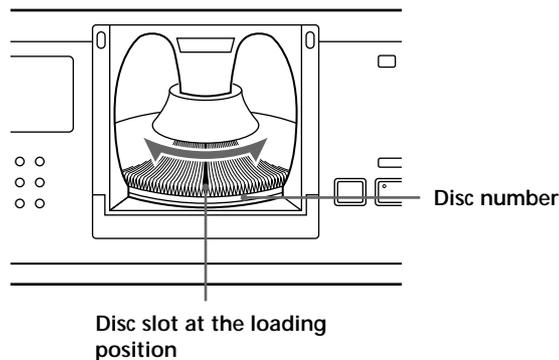
The disc number at the loading position appears in the display.\* As you turn the JOG dial, the disc number changes.
