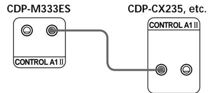
For details on this connection, refer to the supplementary "CONTROL A1II Control System" instructions.
