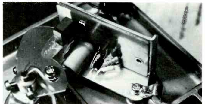
Fig. 5 —Here is the underside of the tone arm, showing the arm magnet near the sensing network. The latter energizes a solenoid which starts the lift and shut-off sequence by releasing a spring-loaded linkage.
