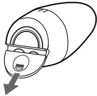
2 Insert two size AA (R6) batteries with correct polarity (+/-), then close the cover.
