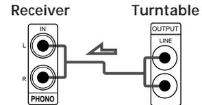
\* If your turntable has an earth lead, connect it to  $\hbar$  SIGNAL GND on the unit to prevent hum.
