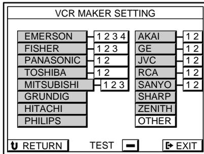
If the manufacturer is not listed, cover the IR sensor on the component to prevent accidental operation during the registration procedure, click OTHER, then go to step 6.
