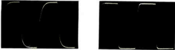
Square-wave response to 10 kHz with full IHF loading (100 K/1000 pF), left; without loading, right.
