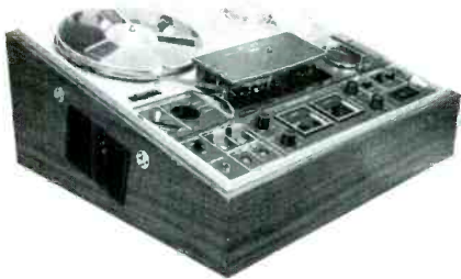
Fig. 1—The 366 remounted in its cabinet for horizontal operation
