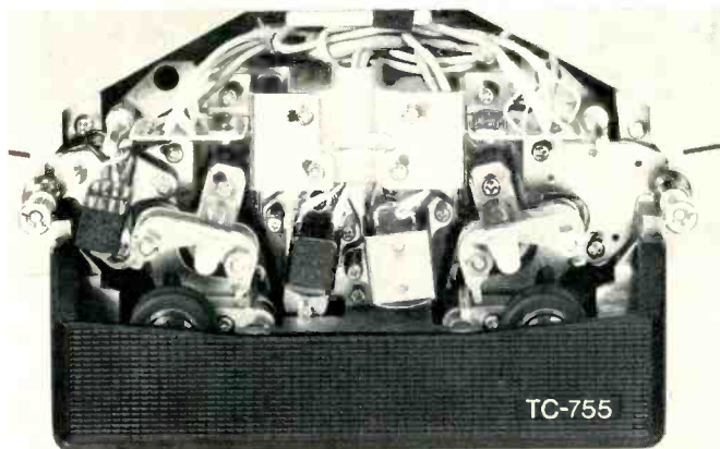
Fig. 1 — Head assembly, viewed from above, with cover removed.
