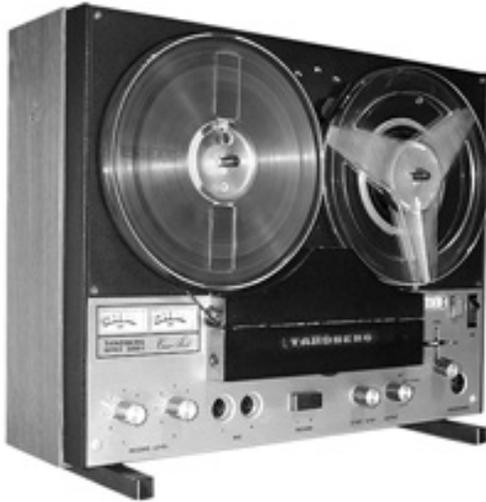
FOR THIS month's review we are examining equipment from the famous Norwegian manufacturer, Tandberg. The recorder is model 3000 X, basically a three-head stereophonic record/playback mechanism, using separate record and playback heads and amplifiers to give full monitoring facilities before and after record.
