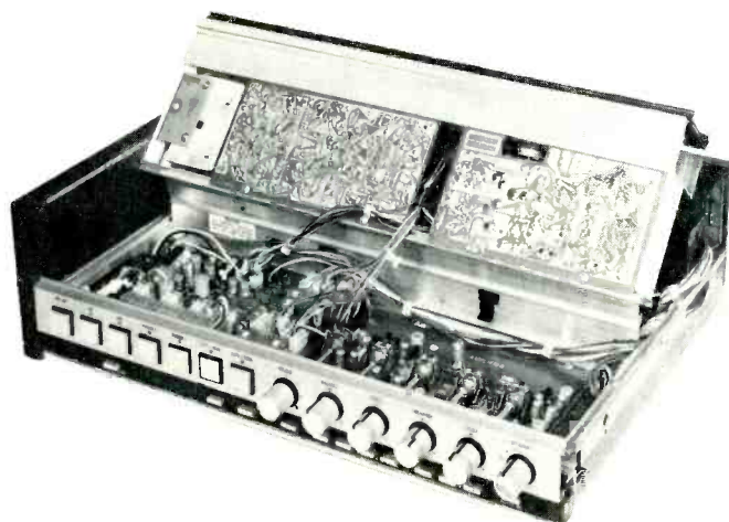
Fig. 3—View with front panel swung up for servicing.
