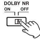
Set the switch to **ON** to record with Dolby Noise Reduction.
