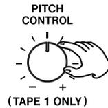
Turning the PITCH CONTROL knob clockwise increases the playback speed and raises the pitch up to +10%.
