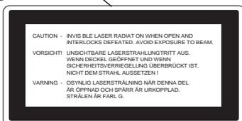
① THIS LABEL IS ATTACHED TO THE PLACE AS ILLUSTRATED TO INFORM THAT THE APPARATUS CONTAINS A LASER COMPONENT.
