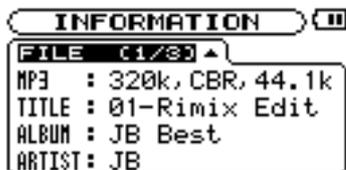
**MP3** File bit rate (kbps), CBR or VBR (constant bit rate, variable bit rate), and sampling frequency (kHz)
