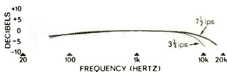
Fig. 5—TEAC playback response to standard recording tape.
