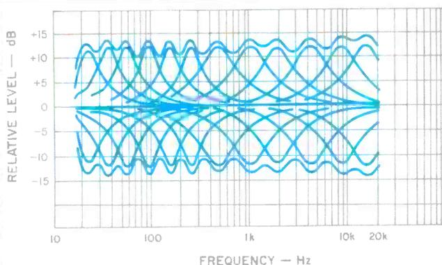
**Fig. 1—Swept frequency responses with each filter at maximum boost and cut and with all filters at maximum boost and cut.**
