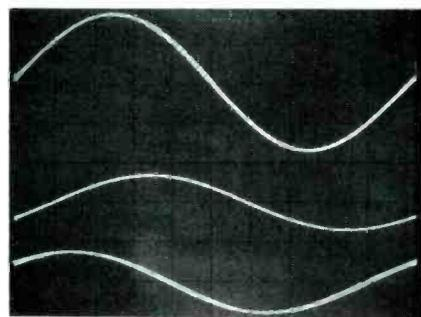
**Fig. 3—**One cycle of a 1-kHz sine wave, showing differing phase and amplitude of maximum boost from each of three filters: 1 kHz (top), 500 Hz (middle) and 2 kHz (bottom). Horizontal scale: 0.1 mS/div. with sweep locked to source.
