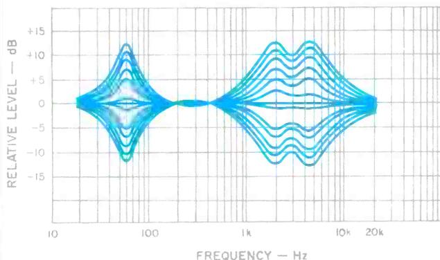
**Fig. 2—Swept-frequency responses with 63-Hz, 2-kHz and 4-kHz filters set successively for 2-dB steps from  $-12$  to  $+12$  dB.**
