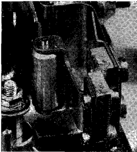
Illustration 1: Rotating tape guide roller in Magnetophon 77.
