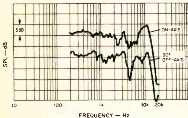
**Fig. 5—Three-meter room response.**
