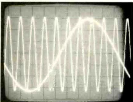
Fig. 8—Phase linearity test, 200-Hz and 2-kHz signals.
