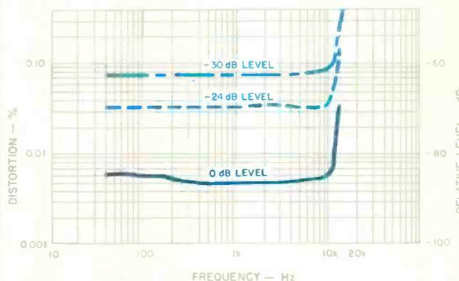
Fig. 3—THD vs. frequency at three recorded levels.
