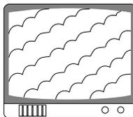
When FM or AM stations are being received, signal noise may be generated if the player is turned on. Turn off the player when not in use. Also, if there is signal noise when receiving radio stations with an indoor antenna, adjust the position or direction of the antenna.
