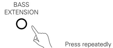
The bass sound is adjusted every time BASS EXTENSION is pressed. Set the button to the desired position according to the atmosphere of the movie you are watching.
