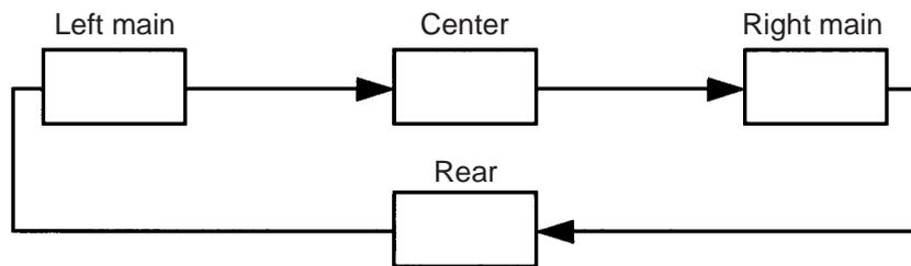
2. Adjust the center and rear level by using the CENTER and REAR LEVEL +/- keys on the remote control so that the sound coming from the corresponding speakers seems to be at the same level as that from the main speakers when you are at a normal listening position. If there is insufficient volume from the effect speakers,
