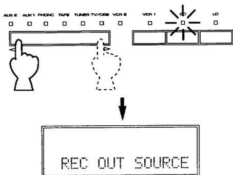
3. Press the REC OUT switch (so that the indicator corresponding to the selected source to be recorded stops flashing).
