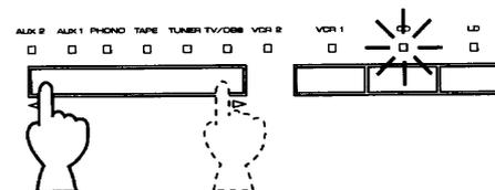
5. Set the tape deck or VCR used for recording to the recording mode.
