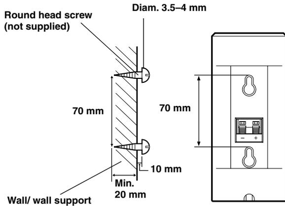
2. Hang the speaker by mounting the holes on the protruding screws.
