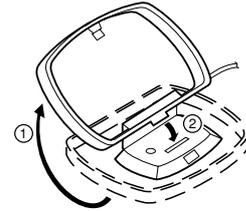
Unwind the antenna wires, then connect them to the AM ANT terminals. Place the loop antenna in a position which yields the best AM reception, or attach it to a wall or other surface.
