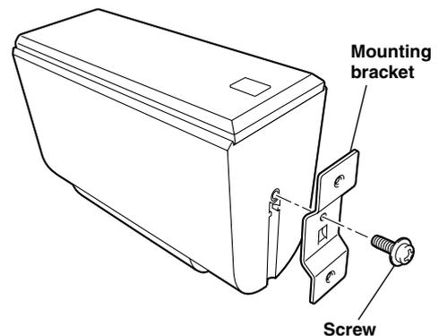
2. Mount the speaker on the speaker stand by using the screw holes on the bracket.
