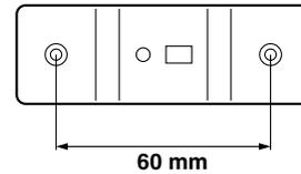
1. Attach the bracket to the bottom of the speaker by using the provided screw so that the convex part of the bracket fits in the grooved part on the bottom of the speaker.
