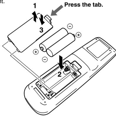
1. Press the tab on the battery compartment cover in the direction of the arrow and remove the cover.
