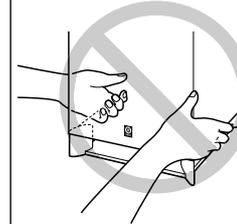
Do not insert your hands into the openings at the lower part of the subwoofer when carrying it. If you touch the inside speaker unit, it may be damaged. Remove the warning label put by the factory setting when using the subwoofer.
