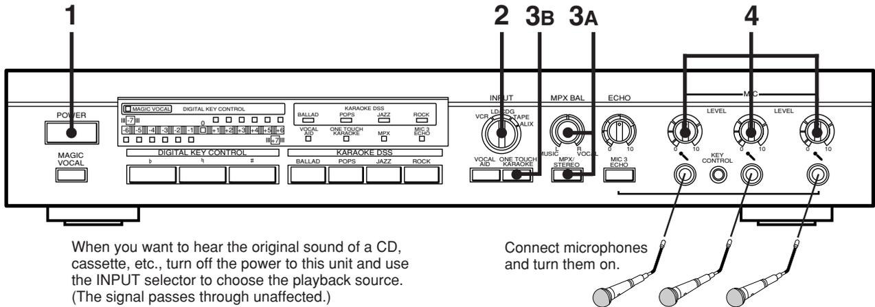
When you want to hear the original sound of a CD, cassette, etc., turn off the power to this unit and use the INPUT selector to choose the playback source. (The signal passes through unaffected.)
