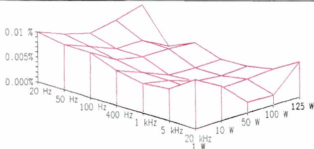
**Fig. 6—Power output vs. frequency vs. THD. Perspective exaggerates the corner point representing 125 watts at 20 Hz, where distortion is only 0.009%. The R-9's distortion remains below its rated 0.015% until above 135 watts (see text).**
