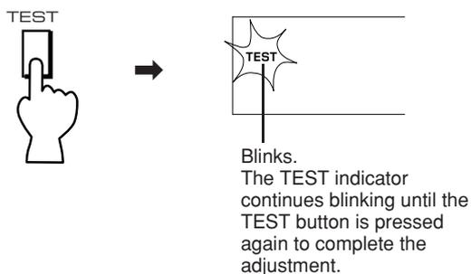
**10** Adjust the BALANCE control so that the sound output level of the left front speaker and the right front speaker are the same.
