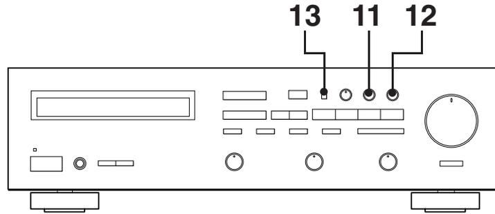
**11** Make the sound output level of the center speaker the same as that of the front speakers with the CENTER level control. (When you selected the PHANTOM mode in step 7, skip this step.)
