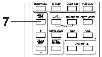
**7** Select the center channel output mode according to your speaker configuration. (Refer to "SPEAKER CONFIGURATION" on page 6.)
