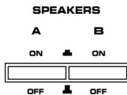
\* If you use two front speaker systems, press both the A and B switches.
