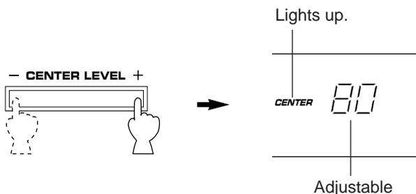
By continuously pressing “+” or “-” on the **CENTER LEVEL** control, the level value changes continuously. However, the value stops changing momentarily at the preset point (80).
