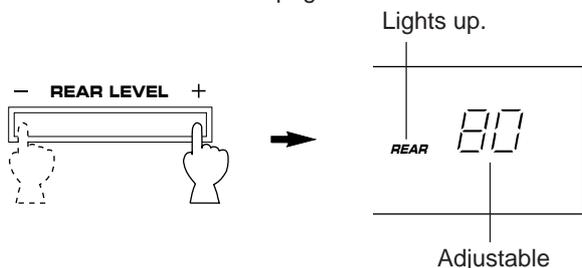
By continuously pressing “+” or “-” on the **REAR LEVEL** control, the level value changes continuously. However, the value stops changing momentarily at the preset point (80).
