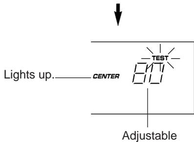
**11** Adjust the sound output level of the rear speakers to be at the same level as that of the front speakers with the **REAR LEVEL** keys.
