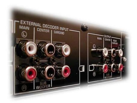
Levels should be straightforward for most: Center, Left Surround, Right Surround, and Subwoofer are adjusted to match the Mains in level. Use your trusty Radio Shack SPL meter and the built-in test tones (or suitable external set such as may be found on Video Essentials) and match the 5 (or 6) channels.
