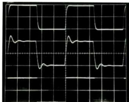
Fig. 5—Square-wave response. Top trace is 10 kHz, with 8-ohm load. With 2- \mu F capacitance across the 8-ohm load (middle trace), ringing is unusually low for an amplifier with no RL buffer. The tilt at 40 Hz (bottom trace) is notably low. Scales: Vertical, 5 V/div.; horizontal, 20 \mu S/div. for top two traces, 5 mS/div. for bottom trace.
